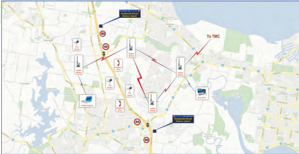
An example of a typical STREAMS Temporary Traffic Management System used during construction of a major road infrastructure project.
