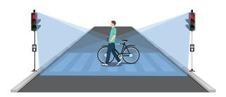
The first part is to detect the pedestrians as they cross the road. This is accomplished by using approved radar on-carriageway detectors.
