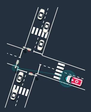
The benefit of the technology is that it helps reduce emergency vehicle travel times whilst enhancing the safety of frontline officers, other road users and the broader community. Every second counts in an emergency and using a smart ITS solution such as EVP to reduce the time it takes for an emergency vehicle to arrive at an incident is helping save lives.
